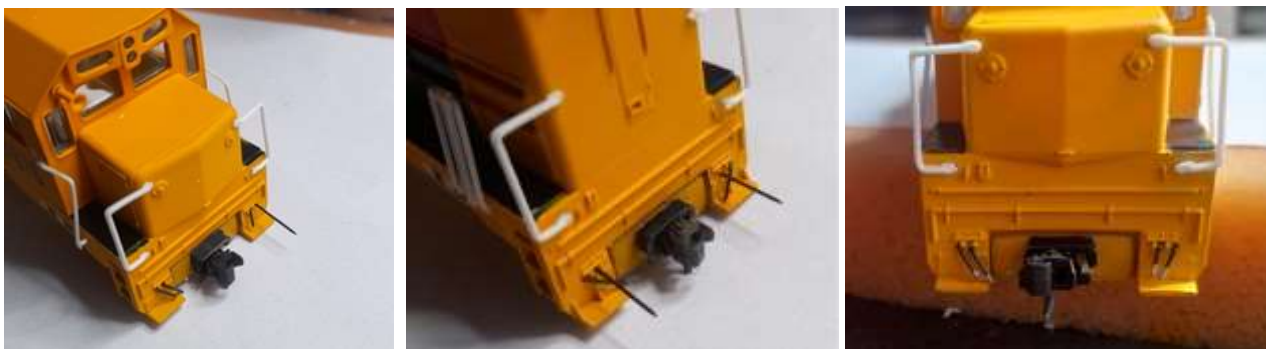
Backing plate applied, and track pins used to secure it, and to make MU hoses
