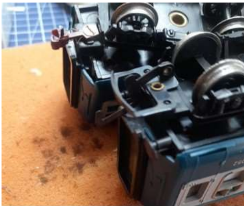
Kaydee couplers added and buffers removed
