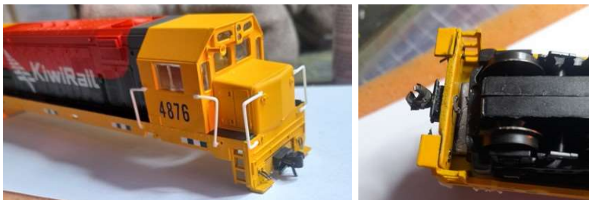
Finished look, and the adaptation of the coupler to fit in the space available
