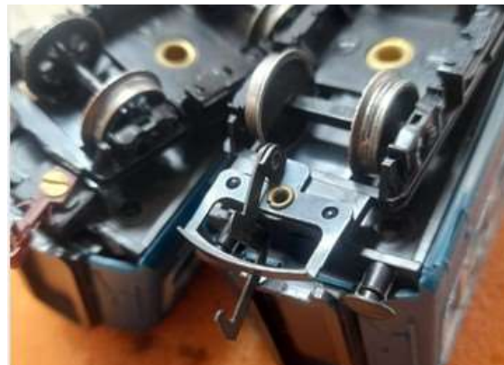
Kaydee couplers added and buffers removed
