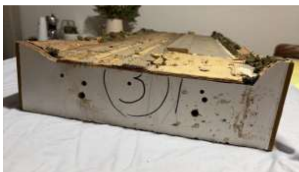
Johnny's old lightweight modules, demonstrating wiring, gazebo pole leg-holes, chipboard usage, and his end-plate profile (Photo credits: Herman Steyn)
