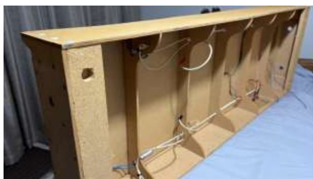
Johnny's old lightweight modules, demonstrating wiring, gazebo pole leg-holes, chipboard usage, and his end-plate profile (Photo credits: Herman Steyn)
