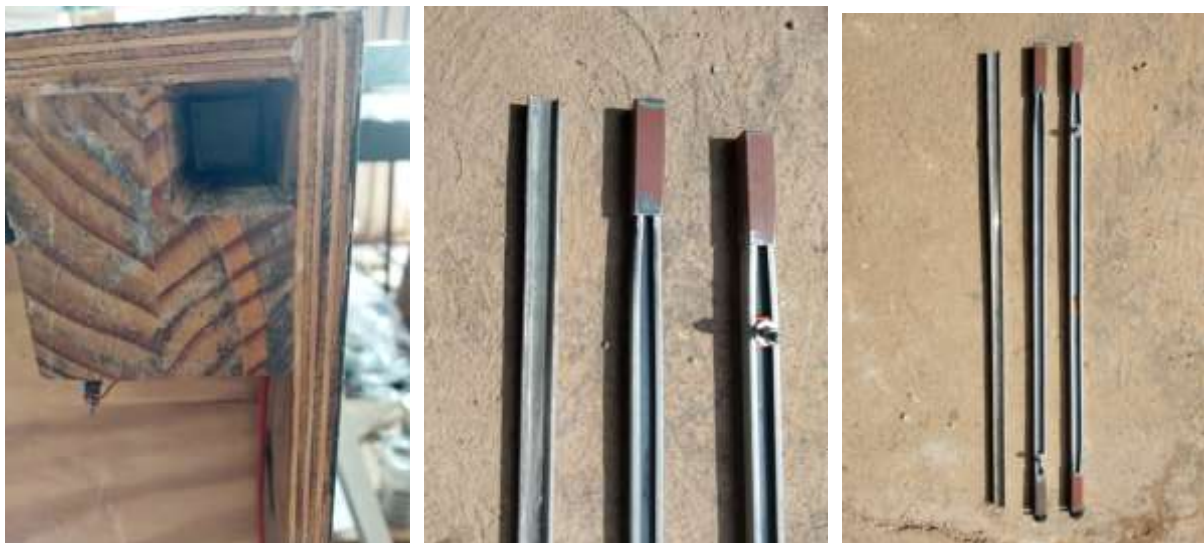
Leg-block (in each corner of each module), and 2x modified (R) vs unmodified (L) legs
