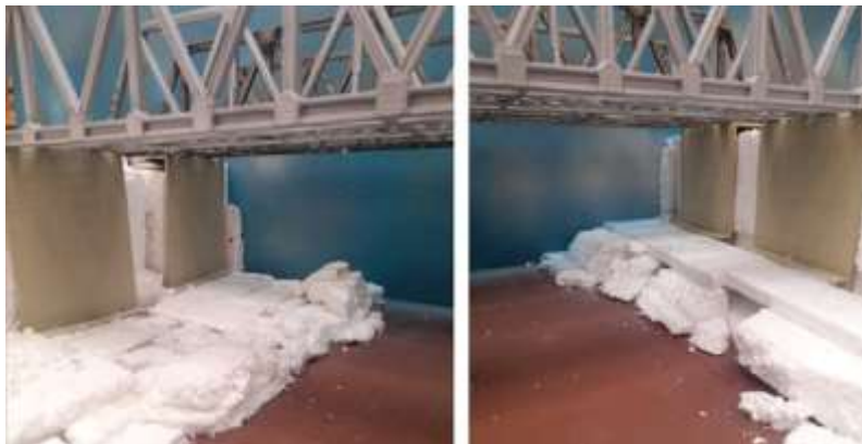
Bridge side supports added into polystyrene and road placement shaped.
