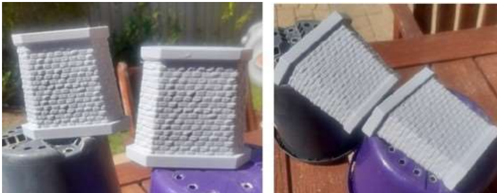
3D-printed bridge supports.
