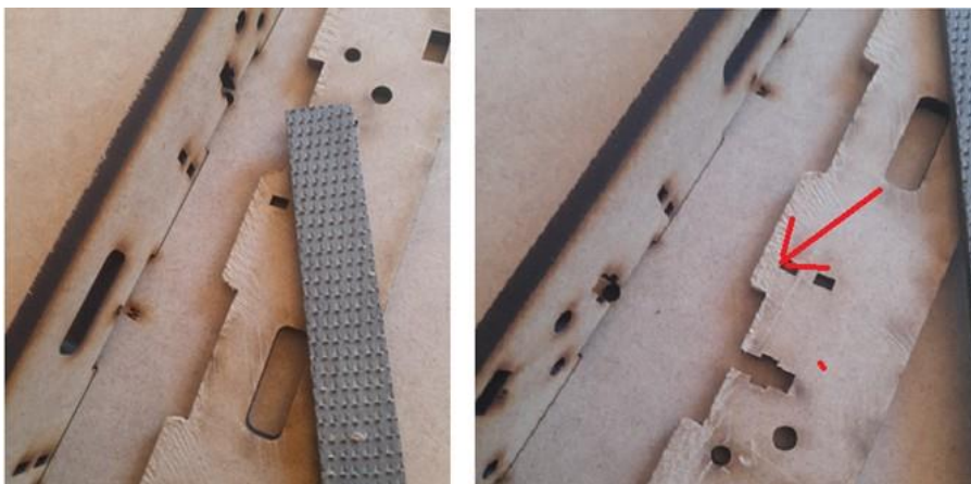
Rasp file used to file and sand the tabs. Arrow shows the level of filing to the body line.
