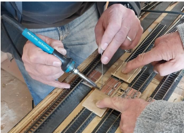
Soldering intact track to PCBoard track-ends
