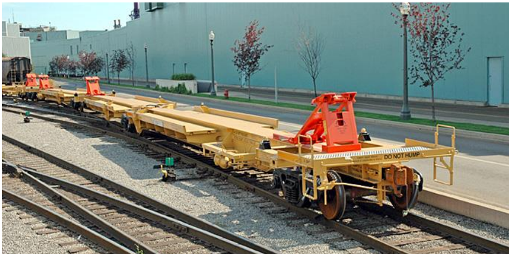
Figure 6: The car that replaced the Front Runner: the spine car. These cars are still in service today.
