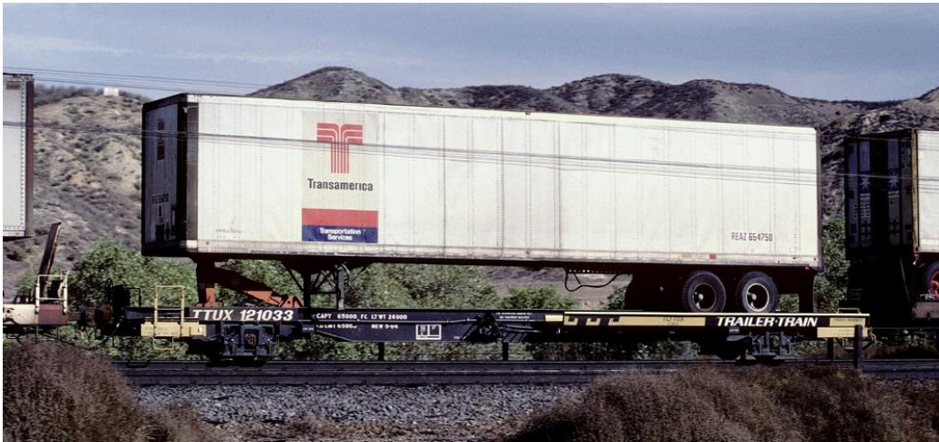
Figure 4: A Front Runner in a TOFC train. The cars on either side are standard 89' flat cars. The difference in heights between the three cars is evident due to the 6" smaller diameter wheels the Front Runner ran on.
