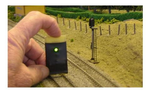
The gadget shown above is a simple device that can tell you immediately whether there is voltage on the rails. Just place it on the rails as shown and if there is power on the rails the green LED will come on. If it does not turn on then the rails do not have power. The brass contacts can also be used to "scrub/scrape" any dirt off the tracks.
